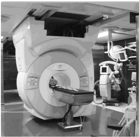
FIGURE 1. View of the ceiling-mounted 1.5-Tesla Espree Scanner (Siemens Wide-Bore 70 cm) adapted by Imris docked to the operating room table in the scanning configuration. Non-MRI-compatible equipment, such as the operating microscope and image guidance display monitors shown in the upper right-hand side of the picture, are moved beyond the 5 gauss line demarcated by the white area on the floor.
